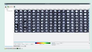
**Crystal Identification** based on fluorescence allows to distinguish salt from protein crystals *in situ*. This can be done fully automated as well, simply by changing the illumination spectrum to near UV-light. This method is also used for identification of initial hits in order to decide which conditions should be selected for optimization.
