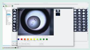
**Image Focus stack** since many plate designs possess lense-shaped wells, crystals might be located at different heights. Some large crystals or disadvantageous bent plates can be even imaged with sharpness when applying an image focus stacking function.
